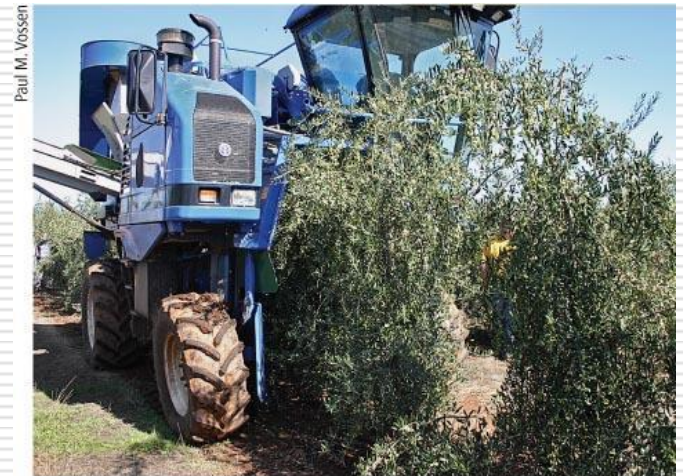
Paul M. Vossen Super-high-density hedgerow planting systems for olives employ over-the-row harvesters (shown, in California).
